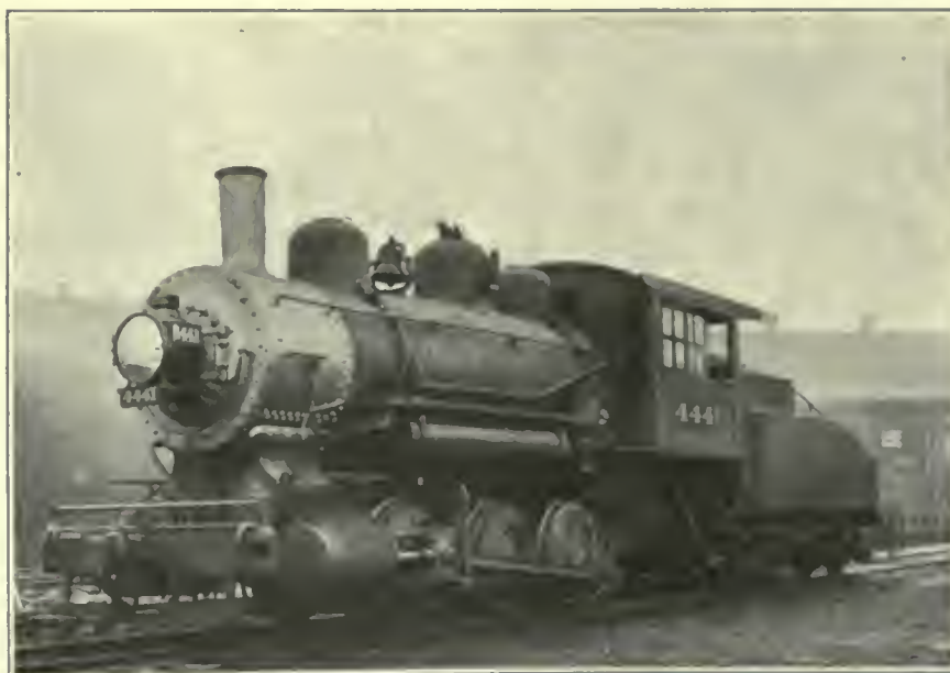
FIG. 388. LOCOMOTIVES. Switching Locomotive of the Six-wheel Type. Lake Shore & Michigan Southern Railway.
